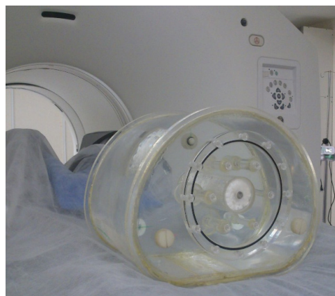
Figure 1. The prepared phantom on the bed of the PET/CT scanner ready for scanning. All inserts filled with F-18 activity.
