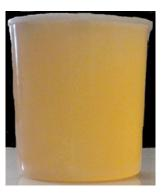
Figure 2. Cylindrical phantom to verify the uniformity of  $B_0$  and  $B_1$ . A cylindrical phantom, with a diameter of 24 cm and a height of 25.5 cm, was made of Plexiglass and filled with vegetable oil.
