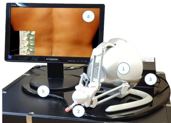
**Figure 3.** Components of the LP Sim hardware including: 1-Falcon 2- Model of LP needle, 3- Processor unit 4- Display and 5- Base platform
