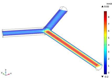
**Figure 6.** Creeping flow profile inside the Y-shape channel
