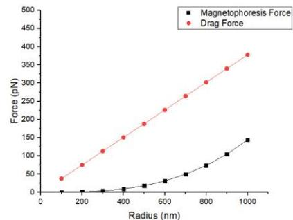
**Figure 9.** The magnitude of magnetophoresis force and hydrodynamic force (pN) with radius variation (nm)
