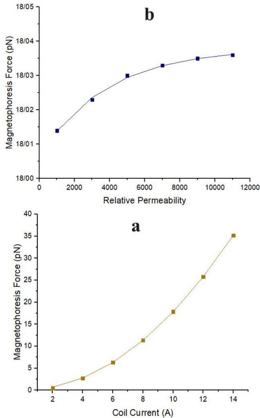
**Figure 10.** a) The magnitude of the magnetophoresis force (pN) for the change in coil current (A); b) Magnetophoresis force (pN) for changes in relative permeability of nanoparticles
