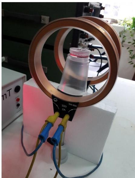
**Figure 1.** Experimental exposure set-up to study the effect of magnetic field on the viability of HUVECs
