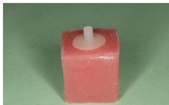
Figure 2. Final zirconia-resin cement samples
