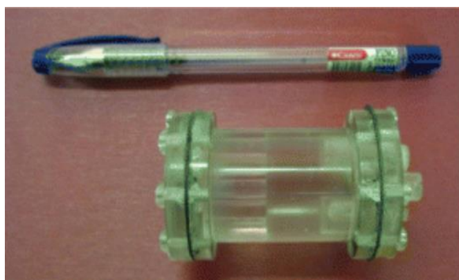
Figure 1. NEMA NU-4 IQ phantom used to assess the reconstructed image quality of the system
