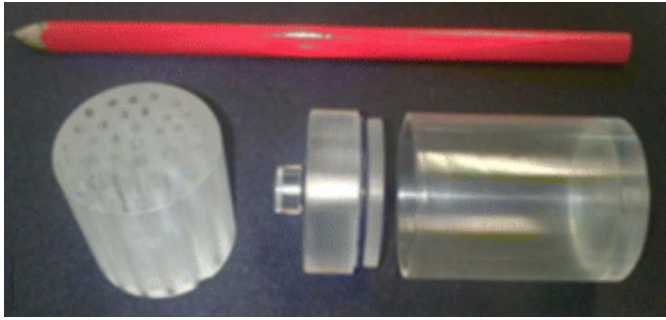
Figure 2. The dedicated in house hot rod phantom designed for tomographic spatial resolution characterization
