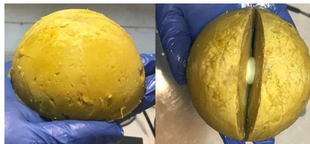
Figure 3. Oil-gelatin phantom of the breast
