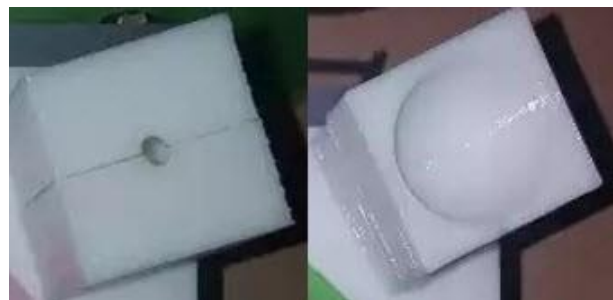
Figure 2. The cube for fabricating tumor tissue. There is a hole on it to inject the mixture in it
