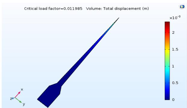
Figure 17. Displacement of design D
