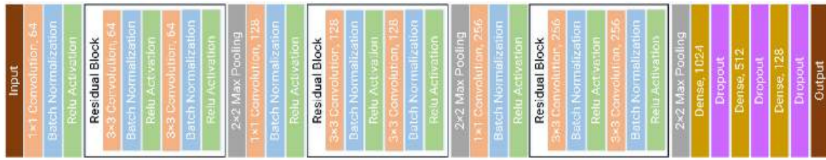
Figure 3. The block diagram of the proposed pixel-based segmentation network
