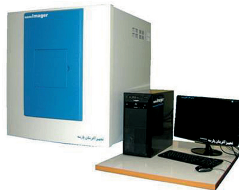
Figure 1. The new Fluorescence Molecular Tomography system; FMT is a free-space system that applied for localizing and quantifying specimens labeled by the fluorescent nanoparticles.
