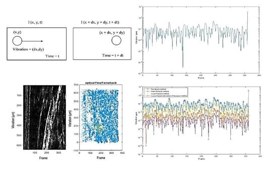
**Figure 1.** a) Definition of optical flow in mathematical language, b) Gunnar-Farneback signal from a vessel wall vibration related to one of the cases, c) An image of vibrations from vessel wall related to one of the samples by Farneback method, d) Four methods of optical flow for a sample.
