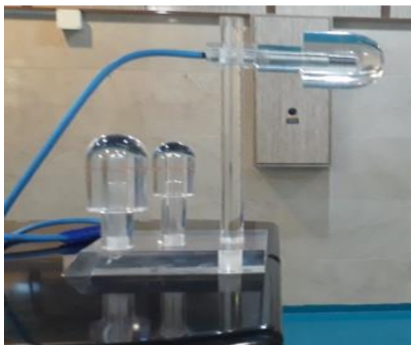
Figure 3. Chamber positioning for the denominator of the couch coefficient
