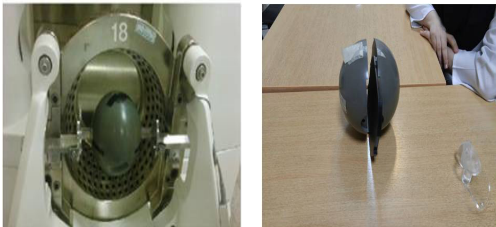
Figure 2. a) Leksell Gamma Knife system with collimator 18 mm, b) Special cassette in the middle of spherical phantom for calibration of TLDs.
