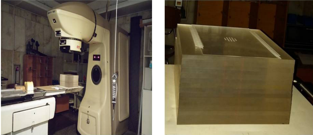
Figure 1. a) Theratron 780-C machine, b) Perspex sheets in the field of radiation.
