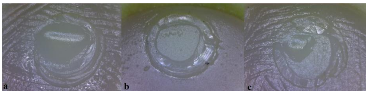
Figure 1. a: Cohesive failure, b: Adhesive failure, c: Mix failure
