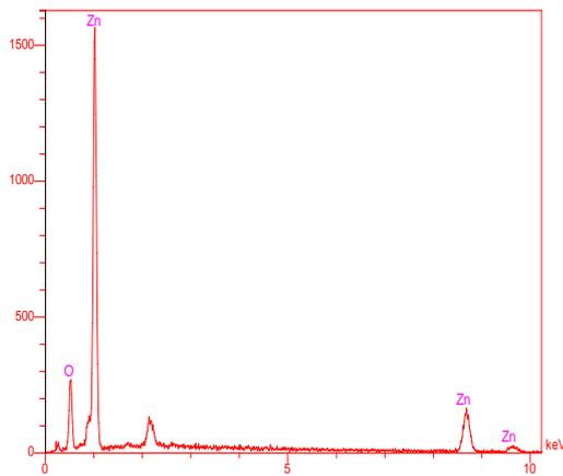
**Figure 4.** EDX spectrum of prepared zinc oxide nanoparticles
