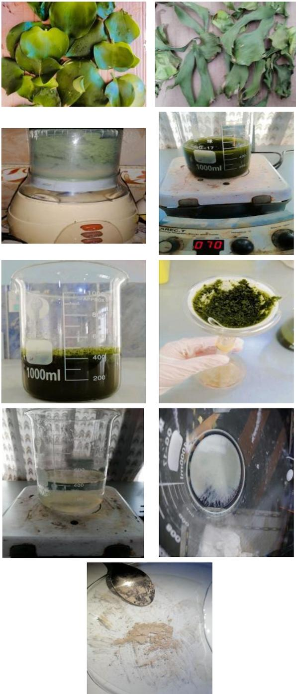
**Figure 1.** The steps of the preparation of zinc oxide nanoparticles using Eichhornia aqueous extract
