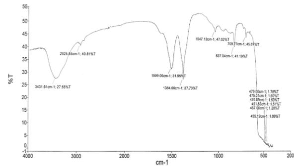
**Figure 5.** FTIR spectrum of prepared ZnO nanoparticles
