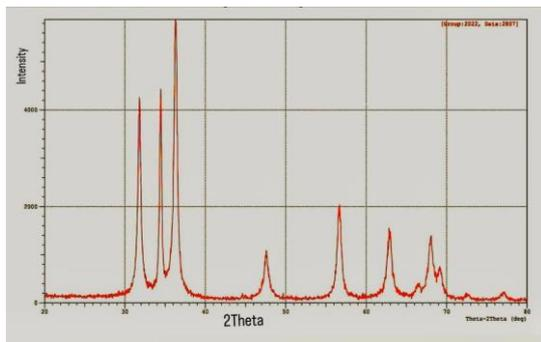
**Figure 2.** XRD pattern of prepared Zinc oxide nanoparticles
